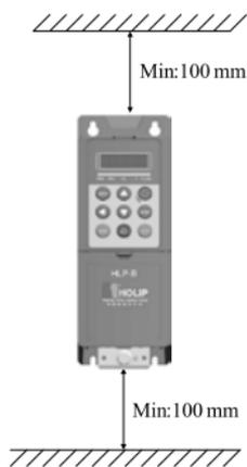
Fig.1 Single installation
