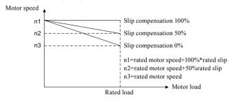
slip compensation on electric driven load
