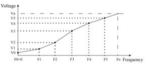
C01.55[0]~C01.55[5] is respective to V0~V5, C01.56[0]~C01.56[5] is respective to F0~F5, Vn is motor rated voltage, Fn is the motor rated frequency.
