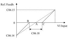
Point A as shown in the figure is the analog value that corresponds to a setpoint that equals 0. It is calculated via analog low, high values and low, high reference/feedback values. After setterminal VI zero dead band, UAB=UAC=C06.18/2. If the VI input is between B and C, the VI reference/feedback is 0.
