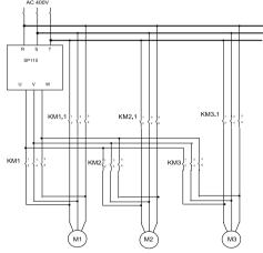
[3] water supply mode 3, the inverter does not go through the relay of the direct drive pump, the other auxiliary pump through a set of relays connected to the grid
