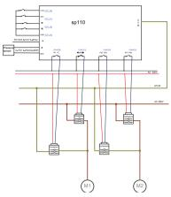
[2] water supply mode 2, inverter up to 4 sets of relays driven by 4 pumps, each pump accounted for A set of relays.
