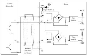
While using this mode, J3 1-2 must be connected (default state: VDD connects to OP). Basic IO board only supports this mode.
